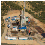
Two drill rigs working on a pad where ten wells have been previously completed
